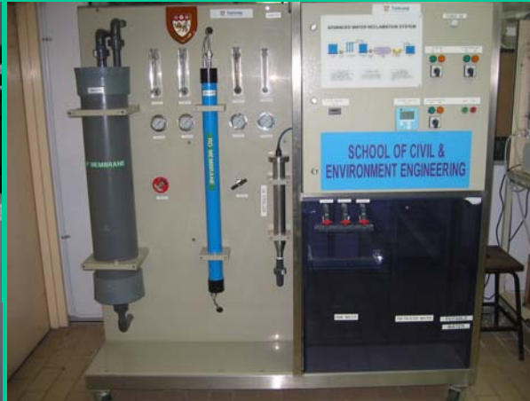
UF/RO/UV Water Reclamation System
